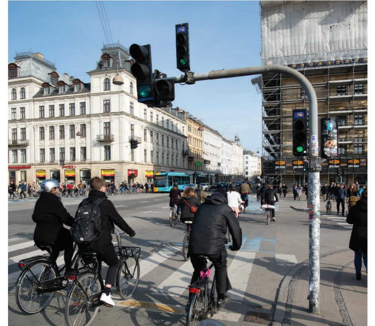
*Dedicated bicycle signals can provide a leading bicycle interval, making cyclists especially visible in the intersection.*
